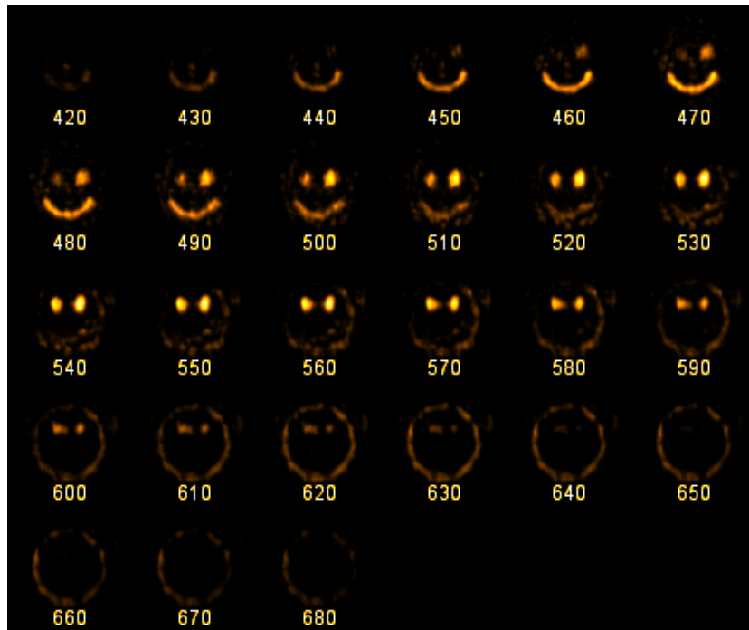
Fig. S3 Wavelength dependent output intensities of the colour smiley APVE. The illumination light was provided by a tunable monochromator. The numbers below the images denote the respective wavelength in nm.
